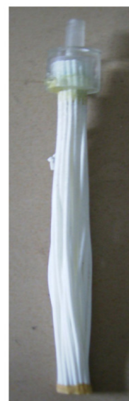
Fig. 1. (a) Schematic diagram of the experimental set-up (1-raw water tank; 2-constant level water tank; 3-reactor; 4-ultrafiltration membrane module; 5-manometer; 6-suction pump; 7-air blower; 8-air flowmeter; 9-air diffuser; 10-discharge valve). (b) Immersed hollow-fiber UF membrane module.
